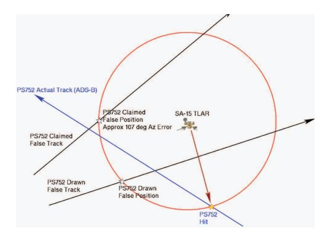
The image above shows the approximate missile system coverage footprint in red and the blue line shows the actual PS752 track based on recorded air traffic reporting data. The black line labeled "Drawn False Track" shows the effect of the miscalibration depicted by the Government in Figure 2. The "Claimed False Track" in black shows generally what one would normally expect from an approximately 107-degree calibration error as claimed in 9.7 p4.
